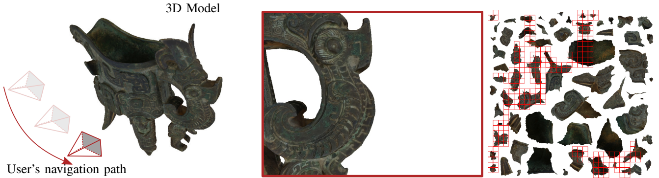
Fig. 2. Example of user's navigation around the 3D model (left), what he observes at a given instant (center), and the corresponding visible blocks \mathcal{V} (in red) in the atlas (right). For better visibility of the blocks, the black background area is turned into white in the atlas.
