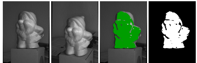
Figure 3. Creation of the mask I , determining the POI region of a scanned surface from the pair of stereoscopic images.
