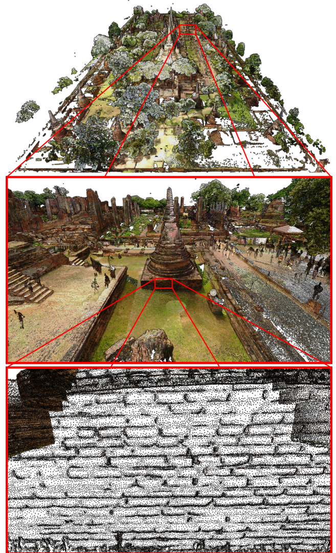
Figure 1: The site Wat Phra Si Sanphet, Ayutthaya (Thailand), resampled with our graph-based approach. The original data contain more than 5 billion points, merging 156 different acquisitions. We are able to represent it with only 2.8% of the original number of points while preserving fine-scale details (such as bricks in a wall over a 40,000m^2 area).
