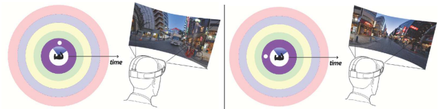
Figure 3: A snap-change re-positions the user in front of another sector of the same scene, in a snap.
