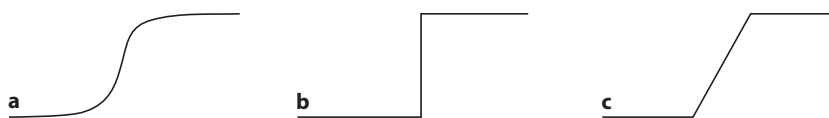
Fig. 1. A sigmoid curve (a), its logical caricature (b), and its piecewise linear caricature (c).
