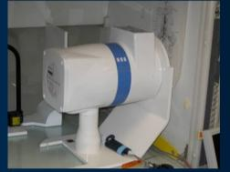
Continuous Nal(TI) crystal : D = 12 cm & thickness = 4 mm
