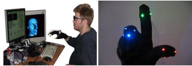
Figure 1: LEFT: User wearing stereo glasses in front of the system . On the left computer, the VRPN server and the two webcam widgets with the colored LEDs detected. On the right computer, the VRPN client with the 3D rendering. RIGHT: Focus on the glove extremities
