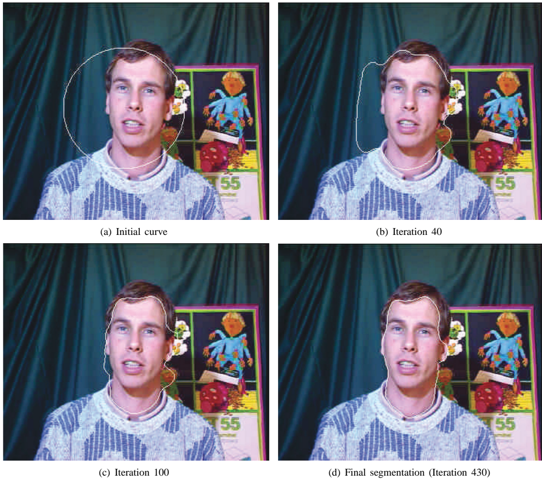
Fig. 9. Evolution of segmentation with the minimization of the criterion (21)
