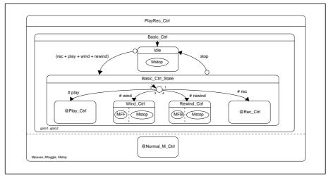
Figure 5. Control of the play-record deck.
