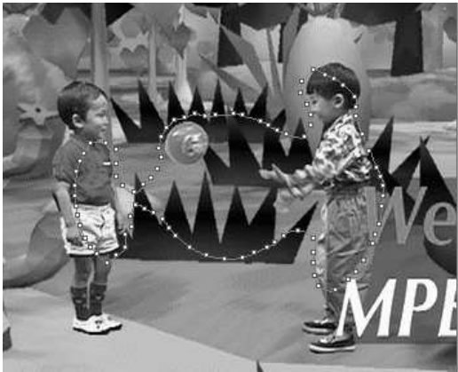
Figure 2: Interpolating Spline Initialization
