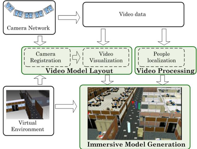
Figure 2. Overview of Virtu4D process
