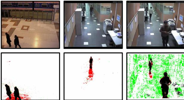
Figure 6. Some foreground extraction results. Foreground elements are in black, shadows are in red and highlights are in green. Left: foreground extraction of the 241<sup>th</sup> frame of PETS’2006 Dataset [14]. Center and right: foreground extraction results in a MPEG-4 medium quality video from our camera network. Right: sudden highlight detection.
