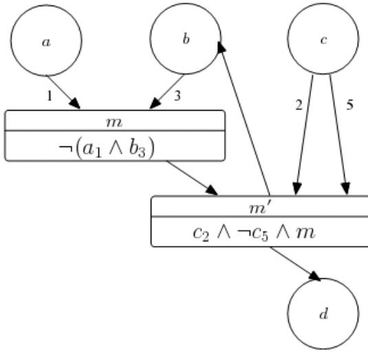
**Fig. 2 Graphical conventions.** This is a RG with 4 variables  $a, b, c$ , and  $d$  and 2 multiplexes  $m, m'$ .  $c$  activates both  $b$  and  $d$  when its concentration level is 2,3 or 4. The complex  $a-b$  inhibits activations.
