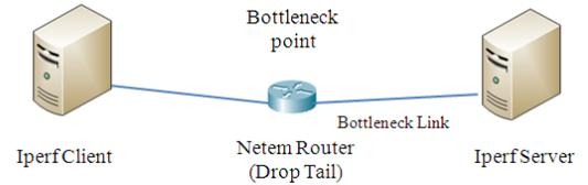
Fig. 3: Experimental network setup
