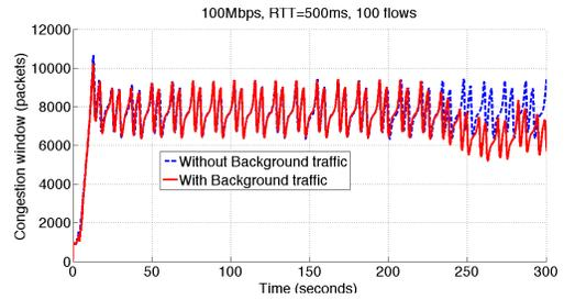
Fig. 8: Time series of window size (packets) with and without background traffic, BS= 1 BDP
