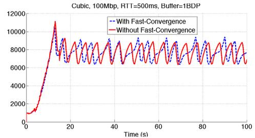
Fig. 9: Time series of total window size (packets) with and without FC, BS= 1 BDP
