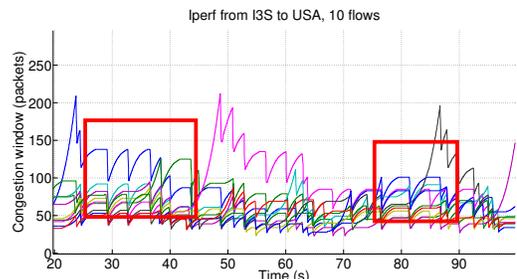
(b) 10 TCP Cubic transfers between I3S and Amazon EC2 data center of Oregon
