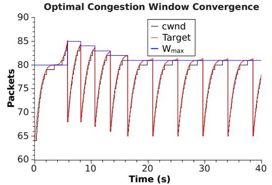
Fig. 11: Converge properties of the optimal congestion window ( $BDP + BS = 80$ ).
