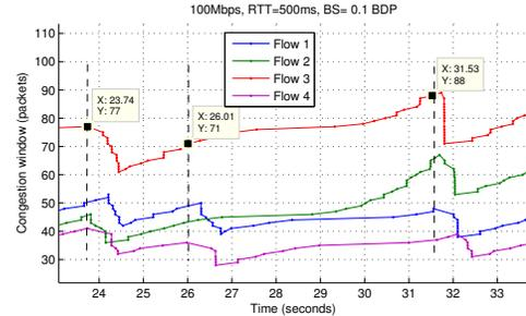
Fig. 13: Cubic leading to a high synchronization
