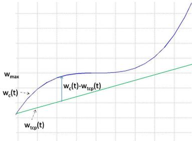
Fig. 2: Congestion window growth of TCP Cubic in Cubic and TCP modes.
